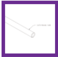
M-Rail 1-1/2" x 1/4" round tube – 20' stock (mid rail)
